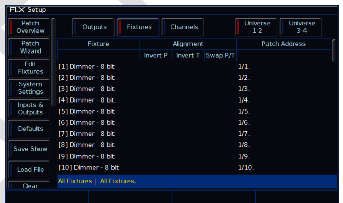
Patch Overview screen in "Fixtures" view.
